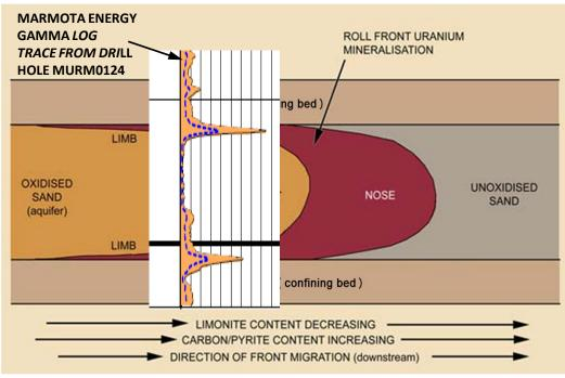
Roll front uranium schematic model cross section overlain by downhole gamma trace from drill hole MURM0124. (Adapted from published sources)
