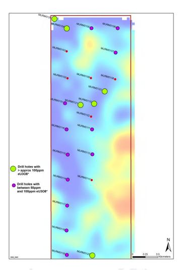
Mulyungarie drillhole locations with eU<sub>3</sub>O<sub>8</sub>\* grades over Bouguer gravity image.
