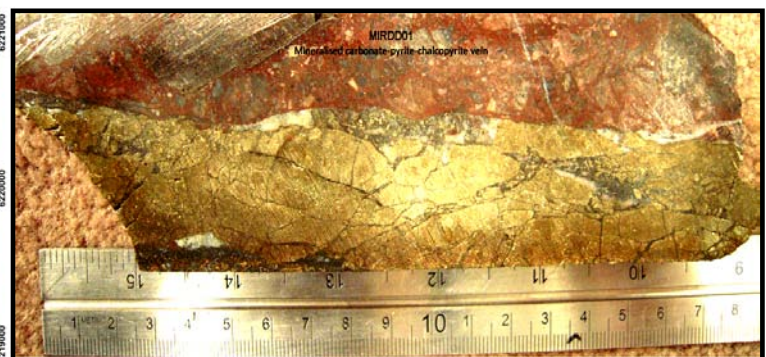
Figure 3: Example of copper mineralisation (chalcopyrite) observed in Miranda drill hole MIRDD01 during Phase 1 drilling.
