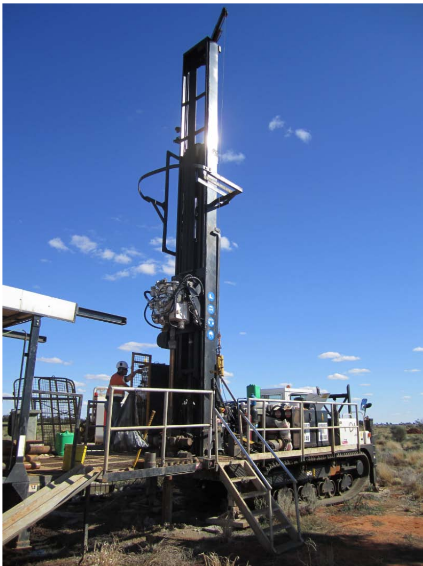
Figure 1: Sonic drilling at Junction Dam – August 2011.
