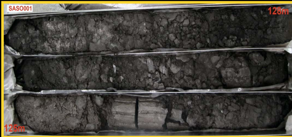
Above. Example of sonic drilling core sample at Saffron.
