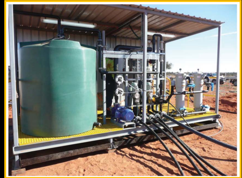
Example of small footprint plant for leach trial: Photograph of Curnamona Energy 's Oban well house for field ISL trial published in July 2010 announcement.
