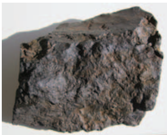
Figure 6b: Example of massive haematite sample from Western Spur
