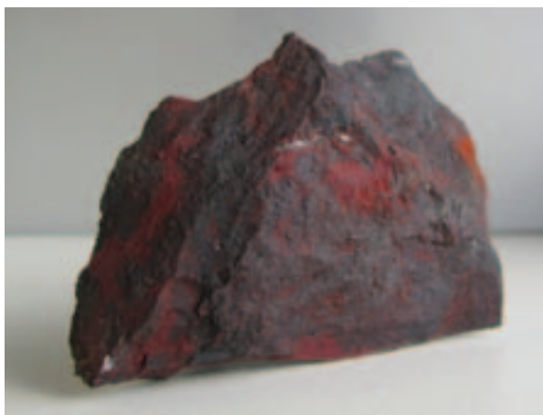
Figure 6a: Example of goethite/haematite iron mineralisation at Western Spur
