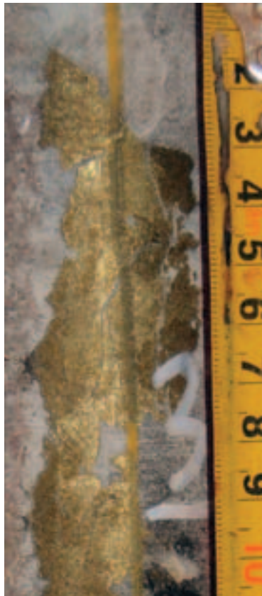
Figure 9a: (left) Example of copper mineralisation (chalcopyrite) observed in Miranda drill hole MIRDD01 during 2010 Phase 1 drilling.
