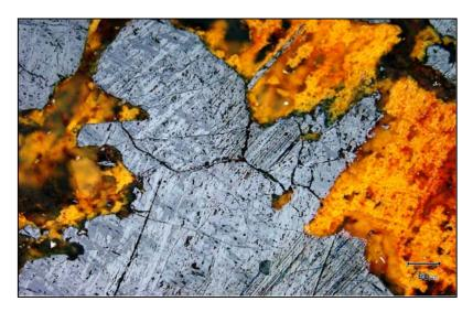
**Figure 5:** Thin section from hematite sample (right). Bright to mid-grey crystals of hematite with diagnostic cross-hatch fabric. Orange-reddish internal reflections within ex-Fe-silicates, oxidised to earthy goethite-limonite.
