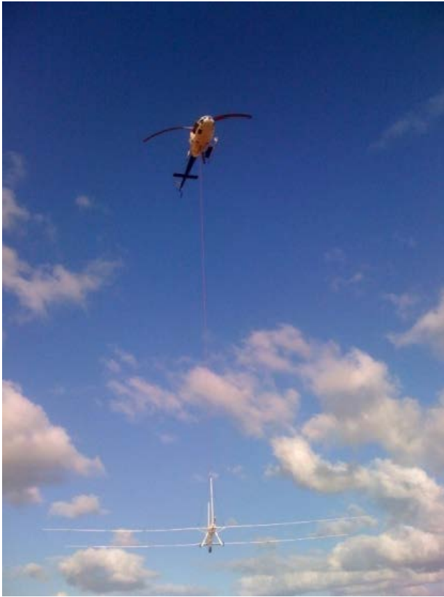
Figure 2 – Heli TDEM survey in progress
