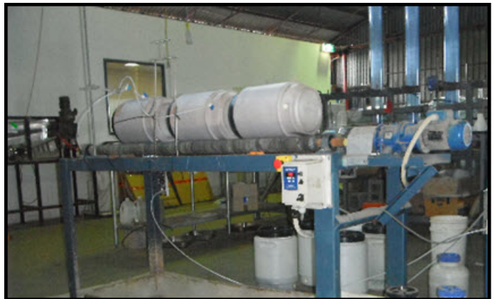
Figure 2: example of bottle-roll leach test
