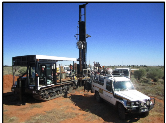
Figure 1: Sonic drilling at Saffron deposit 2011
