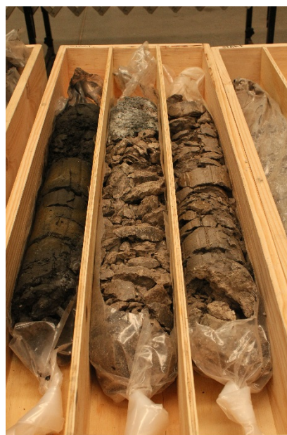
Figure 3; Example of sonic core obtained from drilling at Saffron deposit
