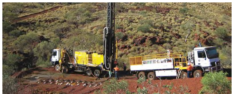
Figure 4: SBD Atlas Copco Explorac 220RC rig on site accompanied by a support vehicle
