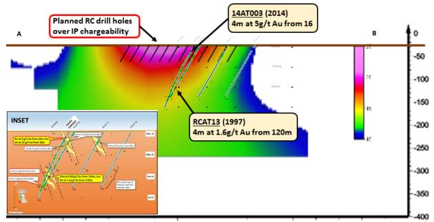
Figure 3 – North-South section across Mars Aurora Tank project showing proposed drill holes targeting IP chargeability anomaly. Inset: Drill section (AON ASX dated: 10/2/2015)
