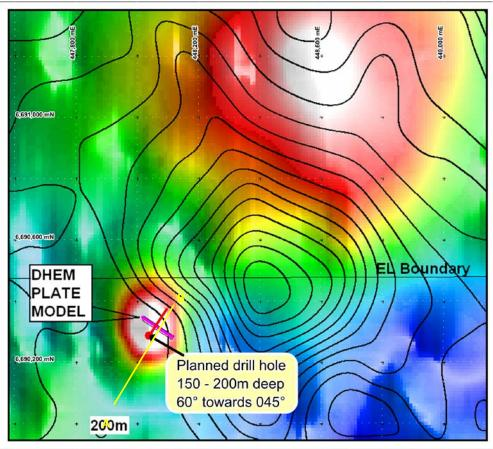
Figure 4 – Bundi MLTEM survey image (Z=ch 25) showing the discrete, high strength EM conductor
