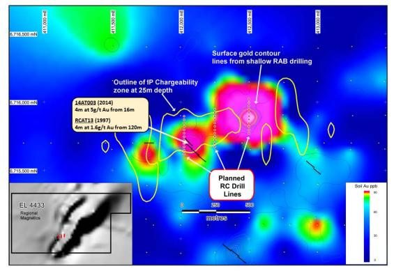
Figure 2 – Proposed drill hole locations at Mars Aurora Tank with outline of IP chargeability high, and coloured contours for gold anomalies in surface RAB samples
