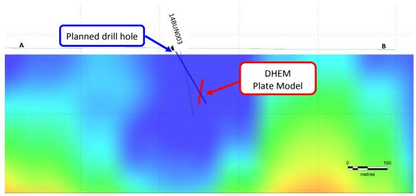
Figure 5 – Northwest facing section of proposed drill hole targeting modelled EM plate conductor on inverted magnetic susceptibility background
