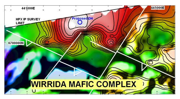
Figure 6 – Plan showing HPX Chargeability Image and Contours draped on aeromagnetics, showing fault boundaries for Wirrida Mafic Intrusive Complex
