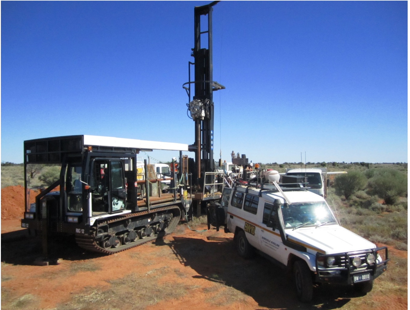
Figure 15: Sonic drilling at Saffron deposit
