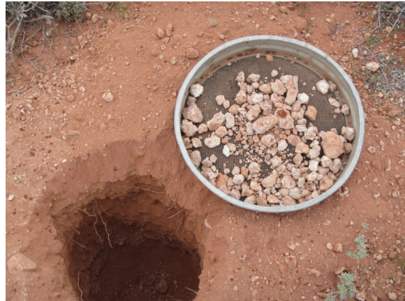
Figure 4: Typical calcrete encountered at the Widgety and Camel prospect included sheet calcrete.
