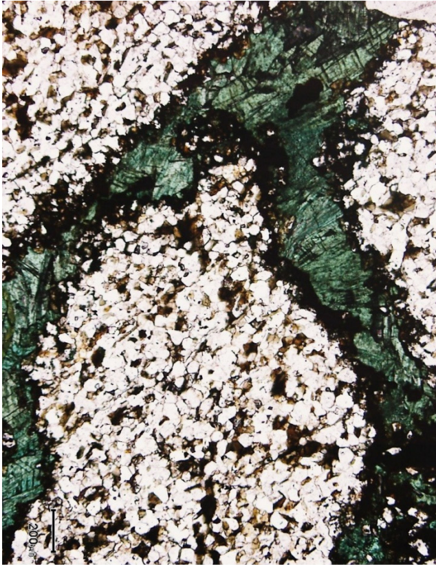
Figure 7a: Hole WMAC007, 25–26m, transmitted light (x50). Branching post-metamorphic veins of malachite in metasilstone.
