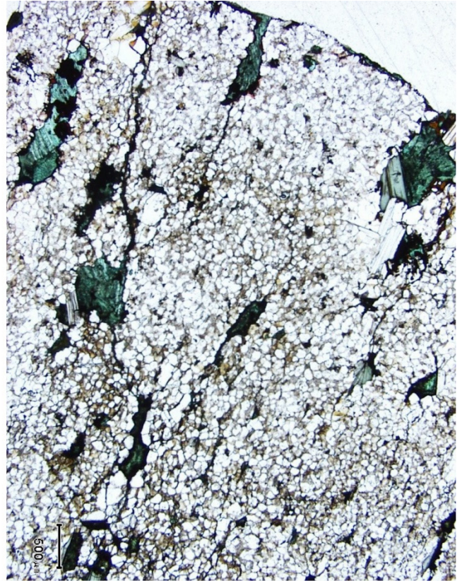
Figure 7b: Hole WMAC007, 25–26m, transmitted light (x20). Small lenses of green malachite occurring sporadically along a weak layering in metasilstone.
