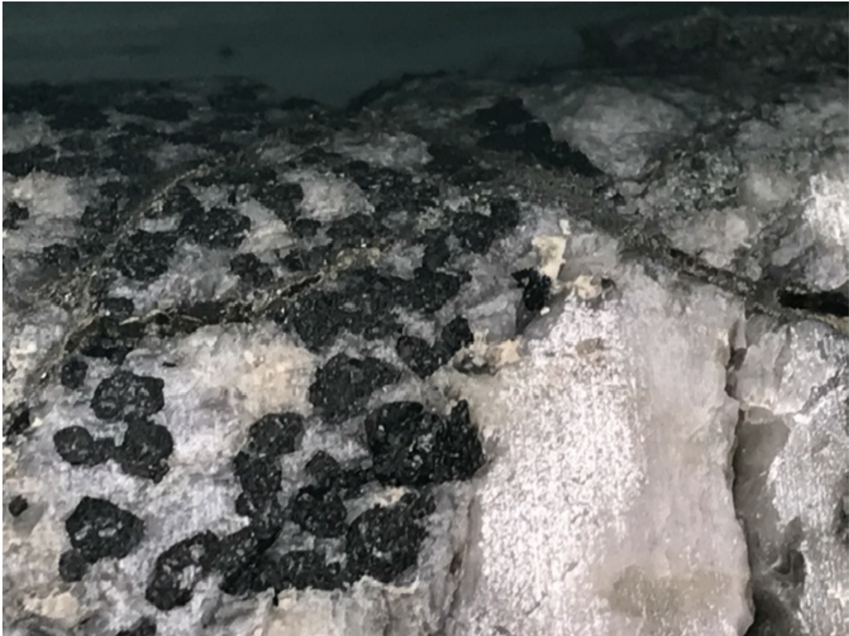
Figure 3: Dense tourmaline crystals on the margin of a quartz vein – Hole 17ATDD002 (from 39.5m)
