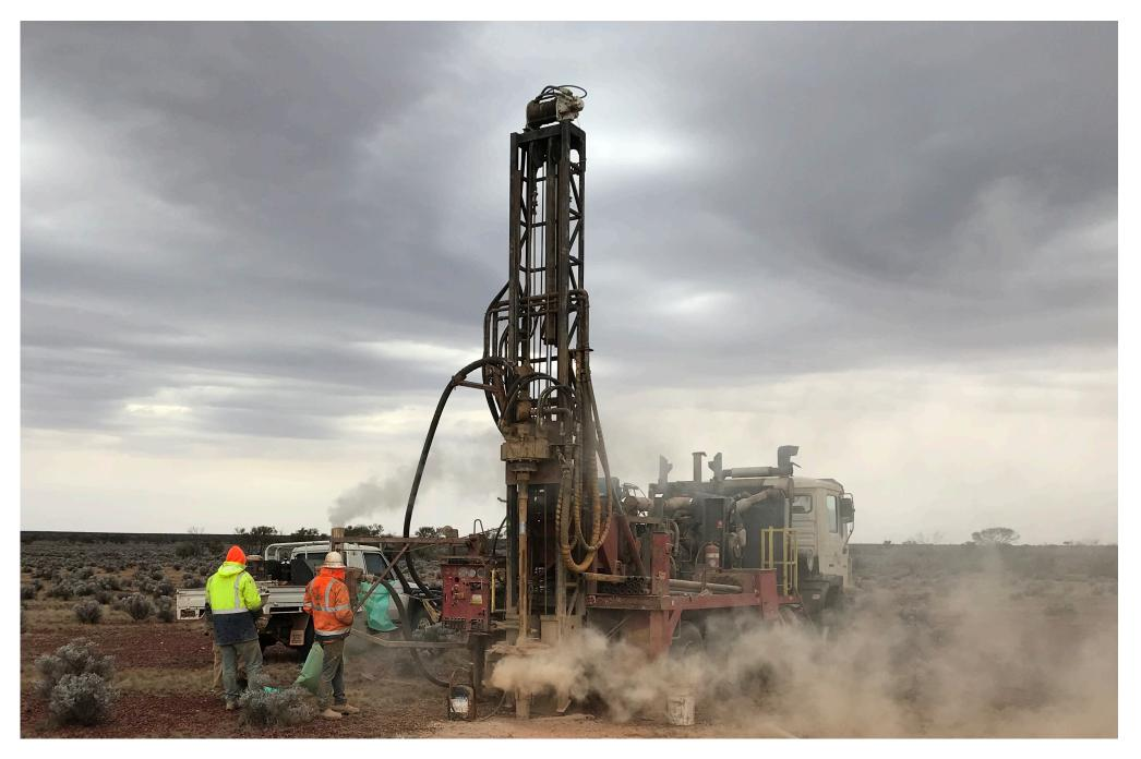
Figure 1: Drilling during program with McLeod Drilling AC rig
