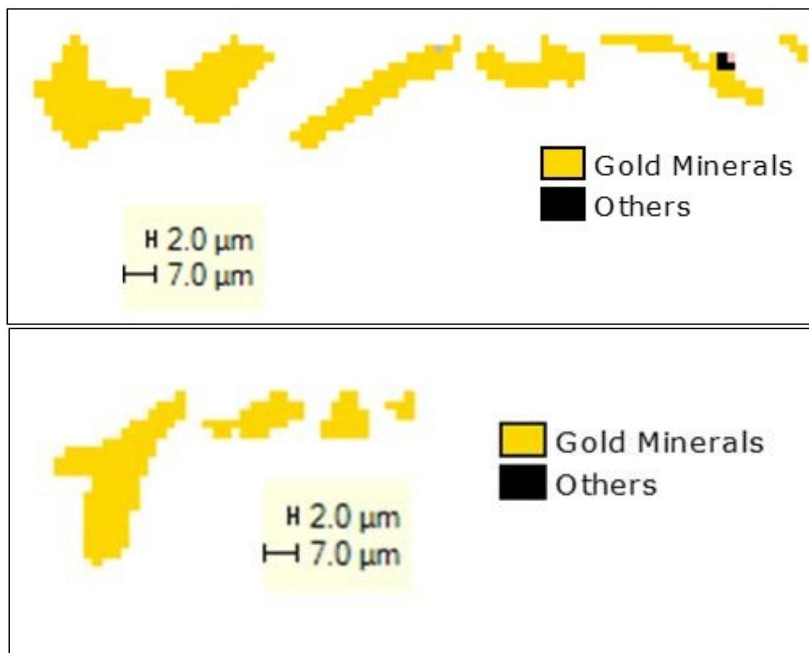
Figure 3: QEMSCAN images showing size and shape of gold grains from supergene (top) and transition zones (bottom)
