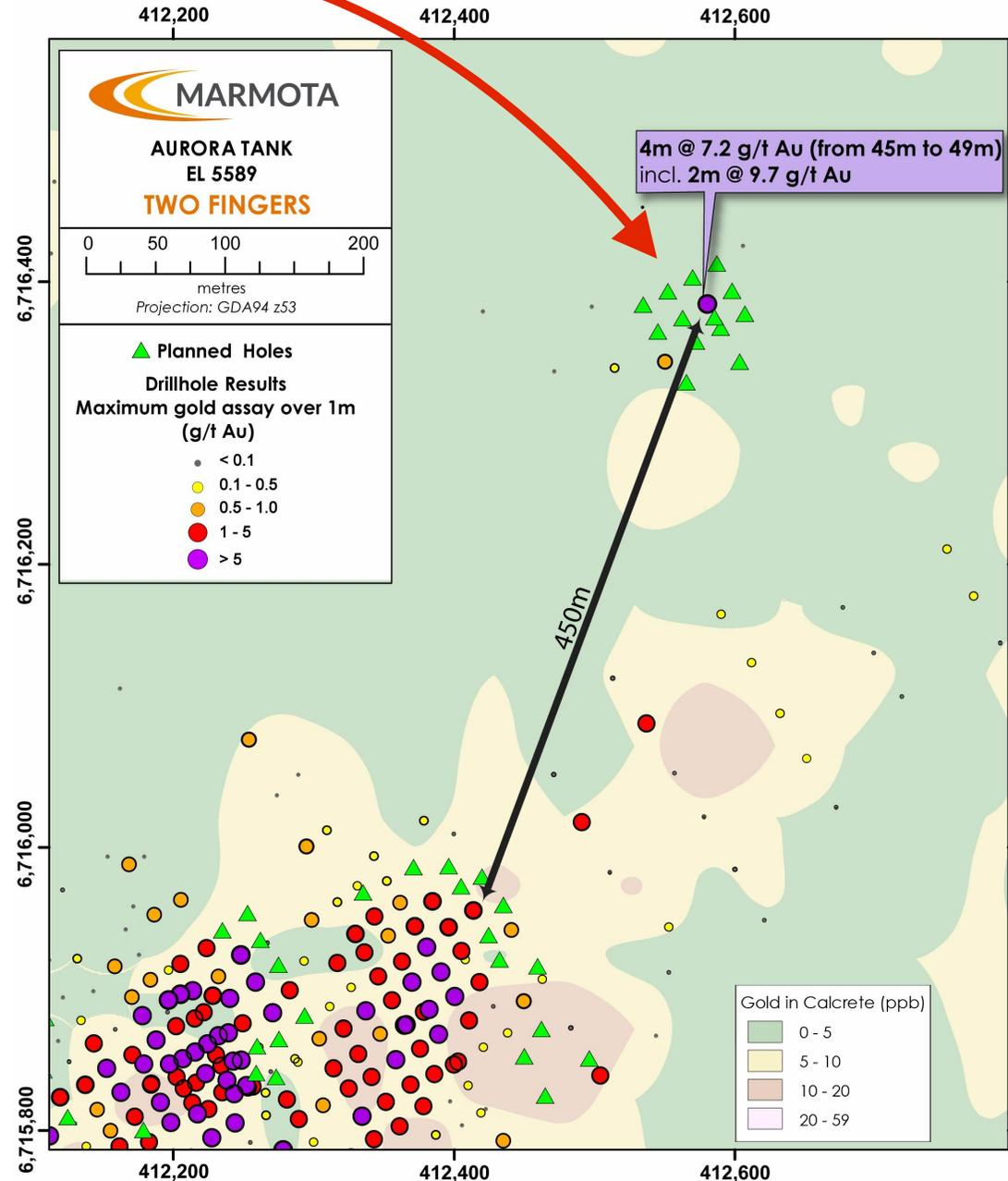
**Fig. 2: Two Fingers discovery Phase 2: 13 planned RC holes** ▲
