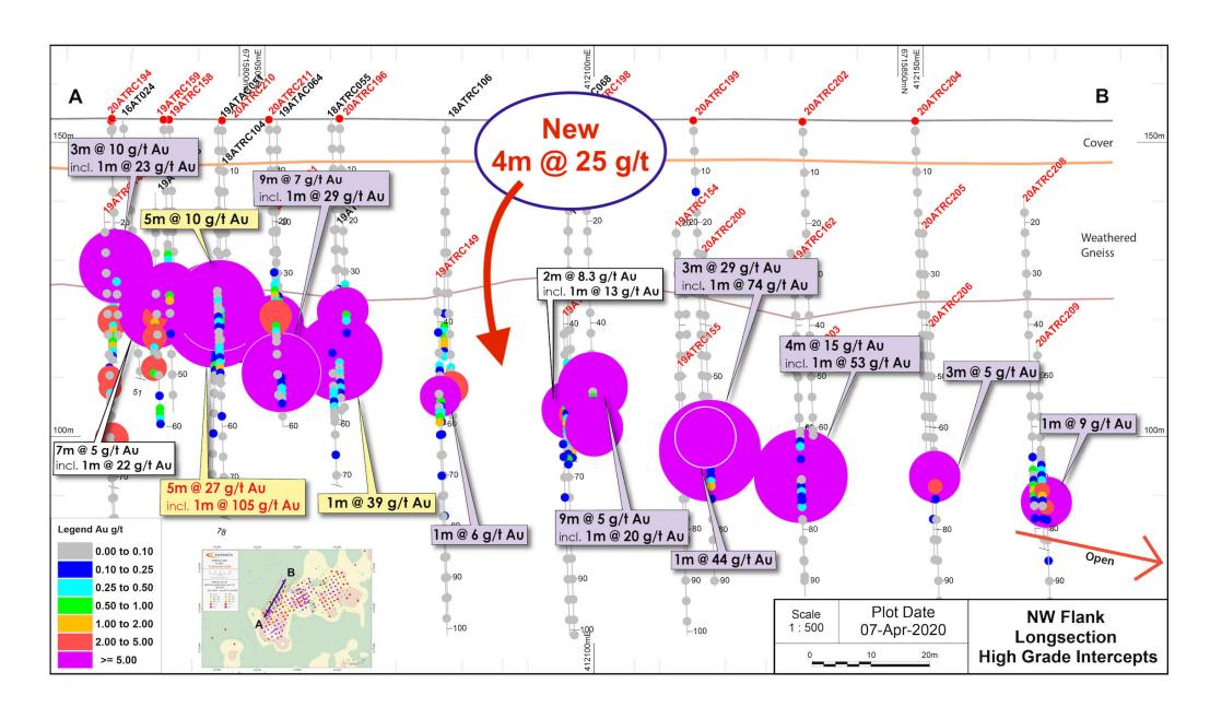
Figure 1: Schematic long-section through NW Flank
