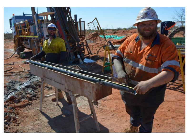
Figure 2: Marmota extends its thanks to the members of the drill crew rig (here with a 2.7m length of core featuring 100% recovery)
