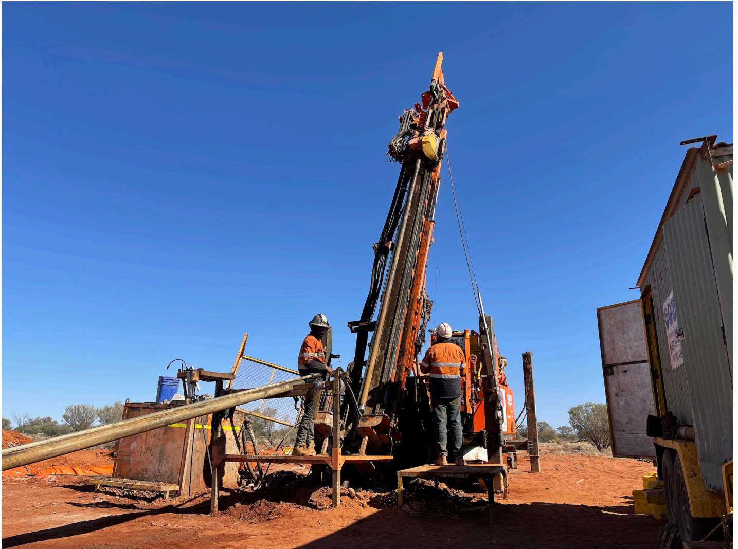
Figure 2: Diamond drilling underway at Aurora Tank ( October 2021 )
