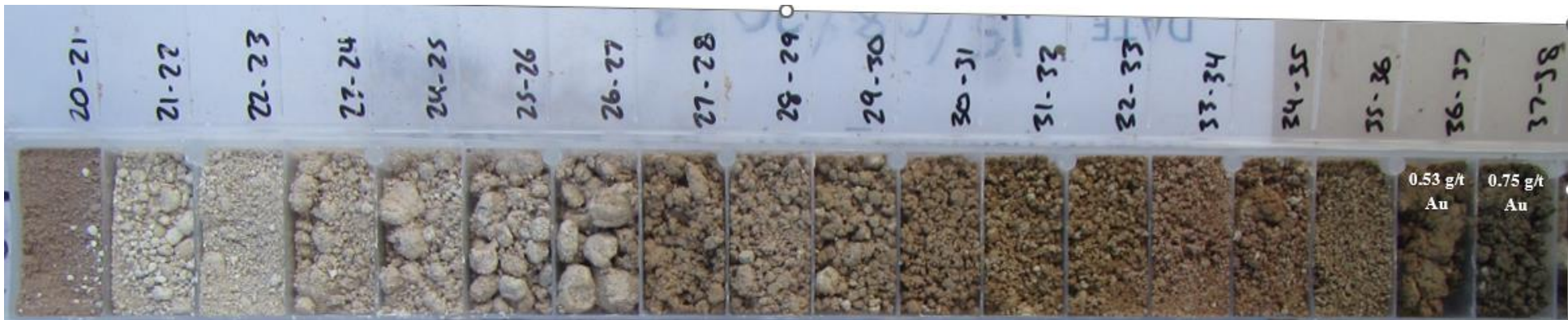
Figure 3: Drill samples collected in chip trays during drilling. Gold mineralisation starts in the last 2 metres, with grade increasing to the end of hole (36m to 38m).
