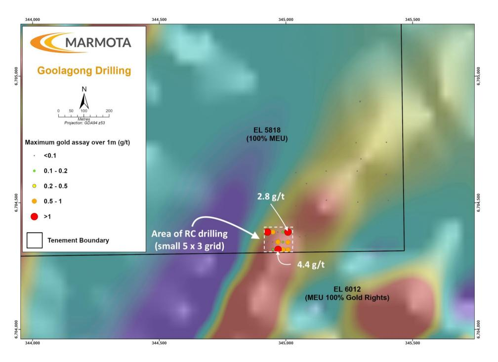
Figure 2: Goolagong on EL 5818: Maximum downhole Au over Total Magnetic Intensity (TMI 1VD) image
